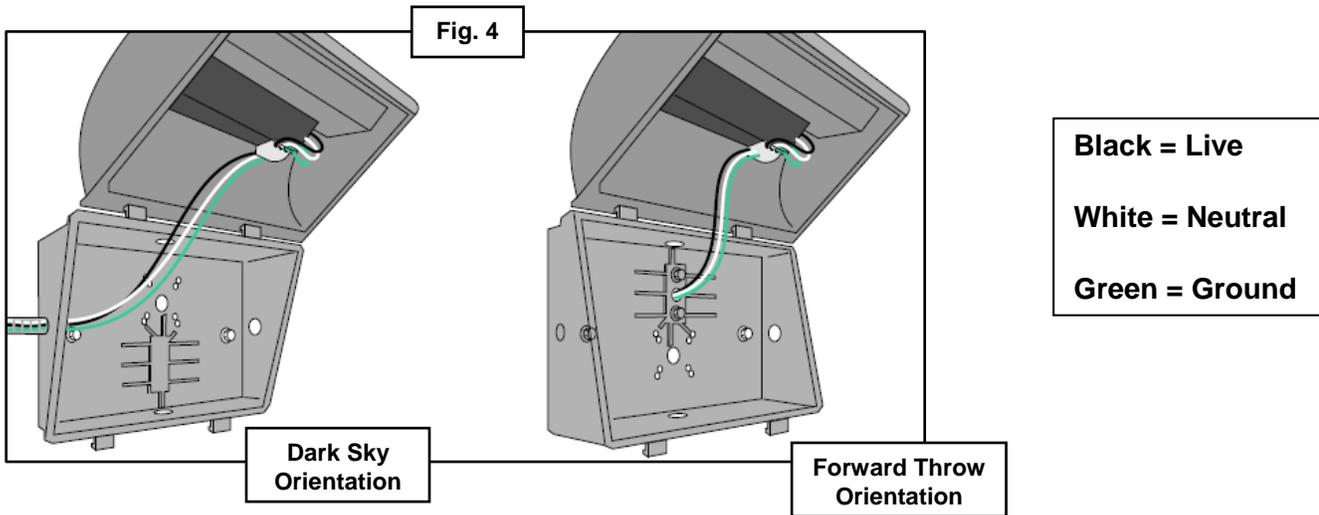
6. Close up wall pack and reinstall screws to secure both sections of wall pack together. Check that seals are all properly positioned to ensure no water enters luminaire.
